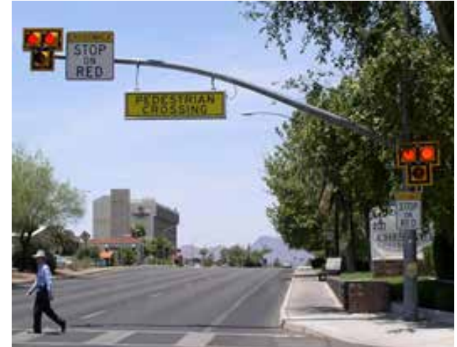
Increasing levels of intensity or investment on bicycle boulevards. Left: Bicycle priority sign on Wilson Street bicycle boulevard in Madison. Center: Mini-traffic circle in Berkeley. Right: Hybrid beacon signal in Tucson
