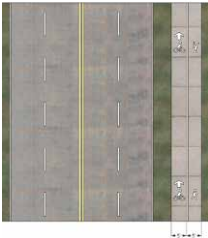
Sidepath sections. Sidepath width and construction standards are similar to those for multi-use trails. Top: Two-way sidepath along an arterial, a typical accommodation on contemporary streets. Above: One-way cycle track concept separates pedestrian from bicycle traffic. Bicycles move in the direction of traffic.
