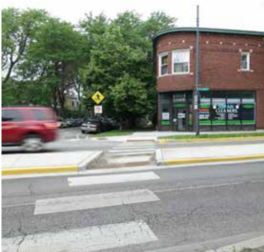
Arterial street crossings for bicycle boulevards and pedestrian corridors. From left: Median installation in Chicago; Crossing median concept for urban corridor by RDG.; diverter island in Los Angeles.
